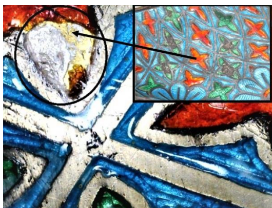
Fig. 7. Digital microscope photomicrograph of the gilding layer beneath the enamel layer.
