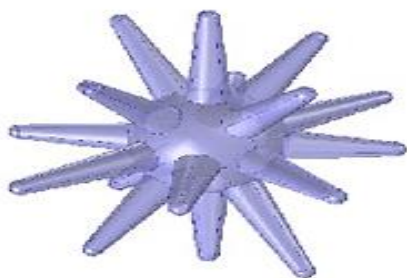
Fig 12: Representation of the nanostar model as defined by the analytical equation for its volume for a numeral of 18 spikes.
