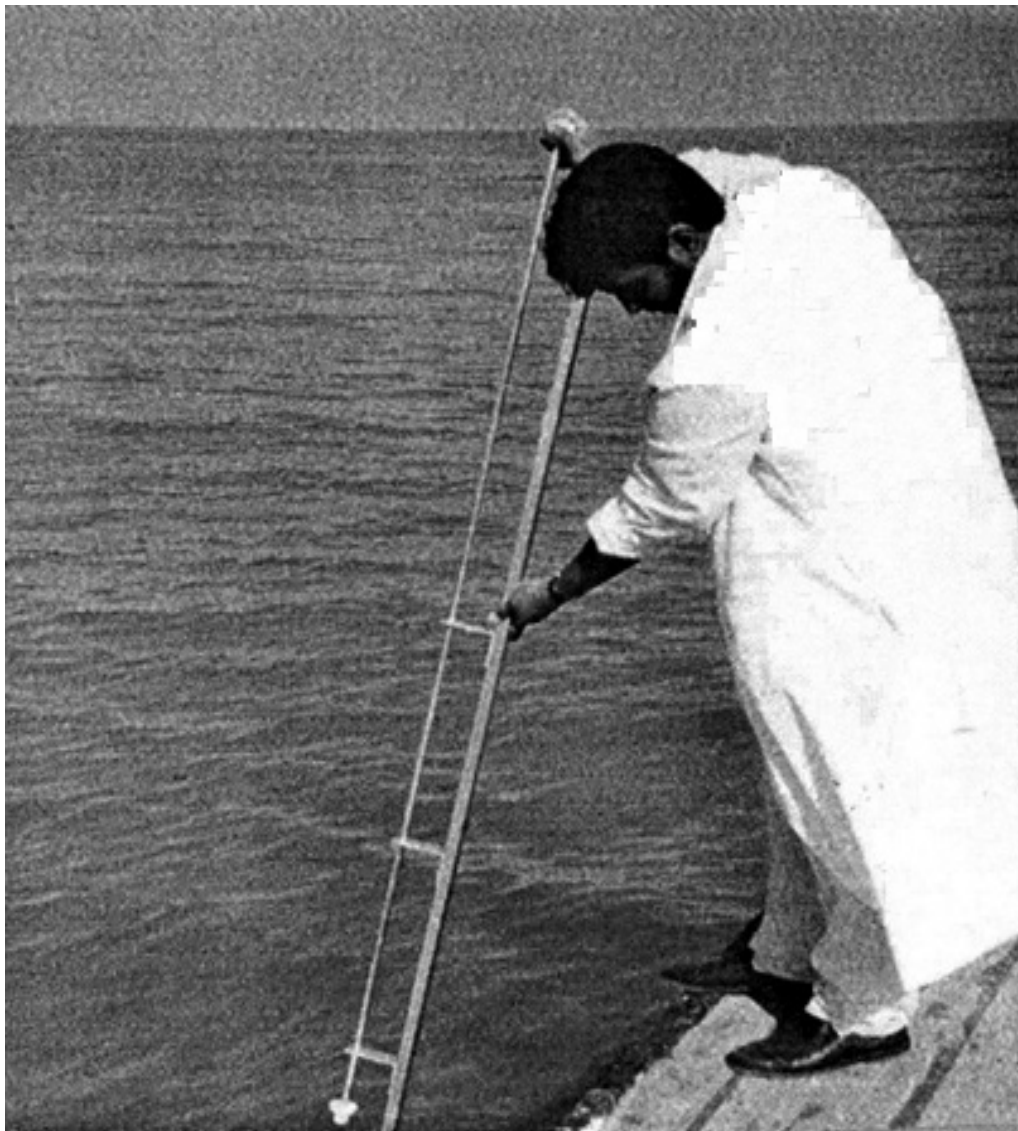
Fig. 3. Subsurface sampling of seawater using sticks.
