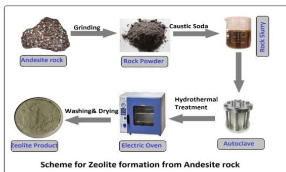
Figure (1): Schematic presentation of the andesite rock-batch Zeolite conversion via hydrothermal method.
