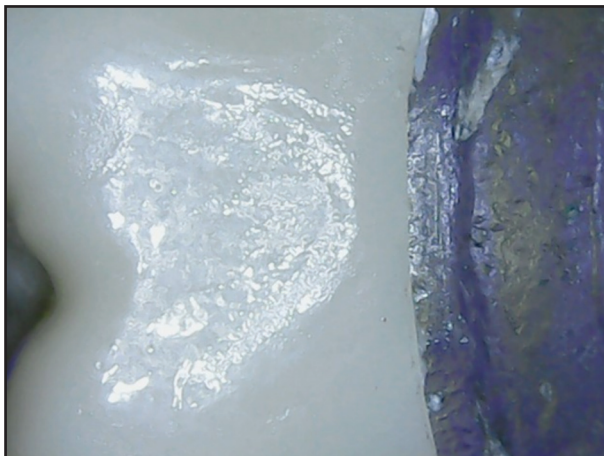
Figure 1 (B): Digital microscopic image for marginal gap of deep chamfer design
