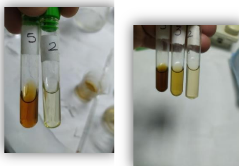
Fig. 2: Difference between two types of soluble hydrolysed sugar after biomass hydrolysis process that as the acid concentration increased the total sugar yield increased indicated as brown colour.
