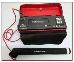
Fig. 2: The Cerescope device used in the present study
