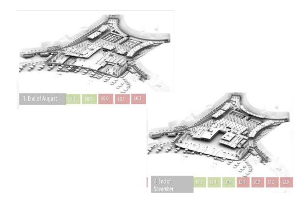
Fig. 10 An extract from the fourth dimension and the development of the project
