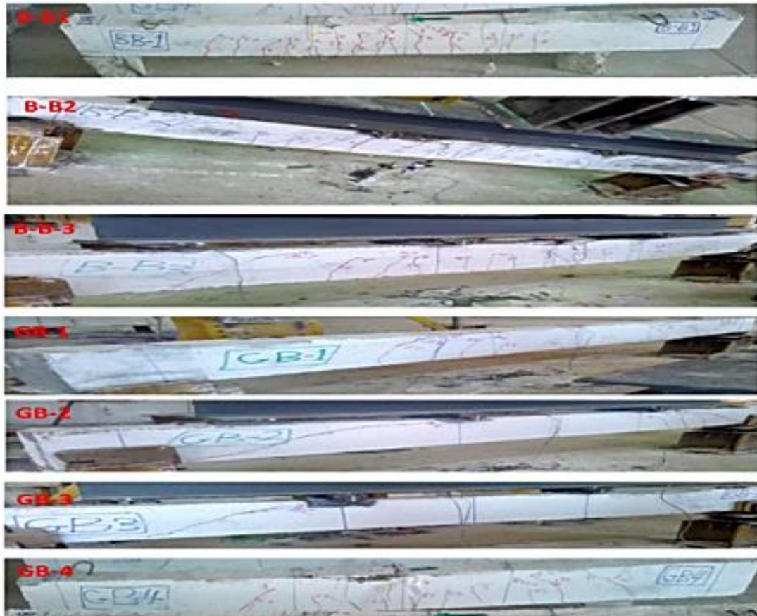
Fig. 8. Failure modes for the different tested beams.
