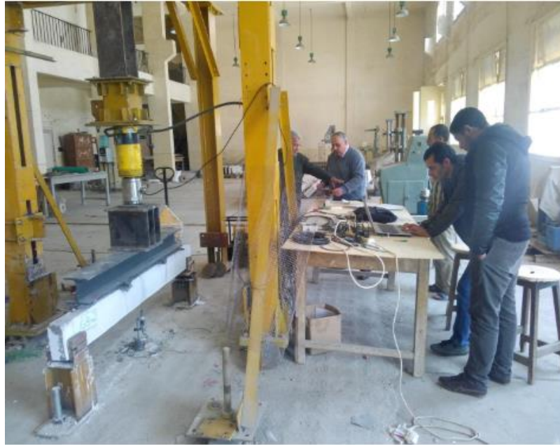
Fig 2. Set up of test beams
