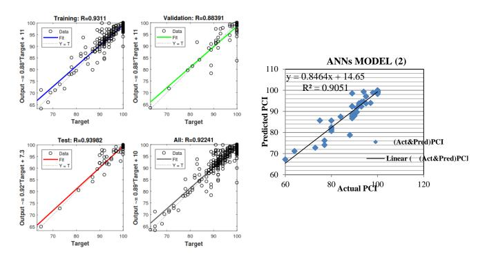
Figure 3: The relation between actual PCI and predicted PCI using Matlab program (The second category of sections- CASE one).
