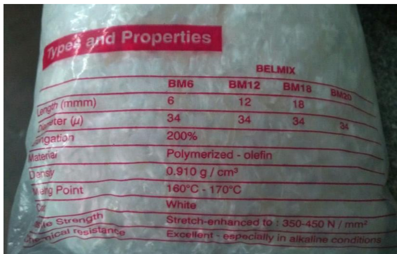
Fig. 2: RHEOFIBRE used in this study
