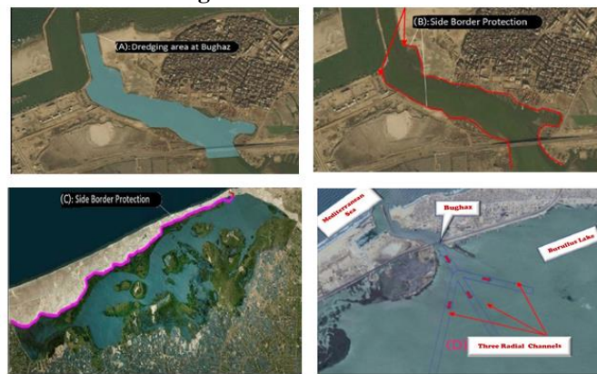
Fig. 2 Burullus rehabilitation project A: Dredging the inlet location, B: Inlet border protection, C: Northwest lake side protection, and D: Inlet radial channel
