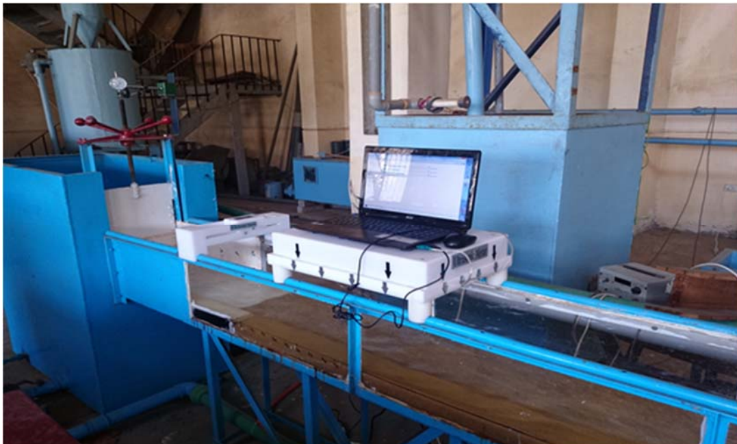
Figure (3) The experimental flume with measuring devices (Ultrasonic devices - multi spots)
