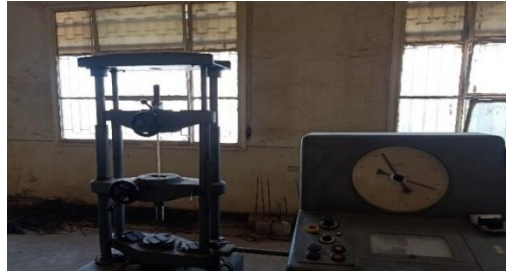
(a) GFRP tensile Strength method machine
