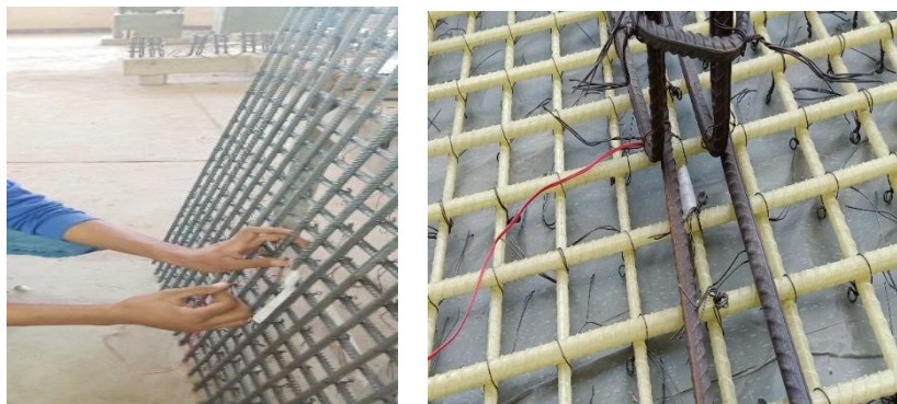
(a) Reinforcement electrical strain gauge location
