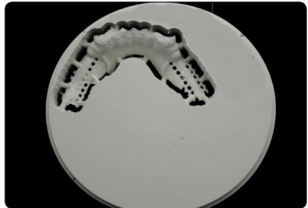
Fig. (3): Milled PEEK framework before cutting for group (I).
