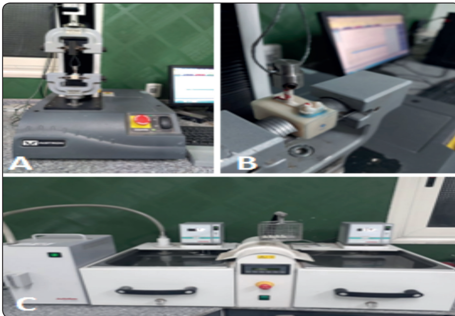
Fig. (5) A Instron Universal Testing machine, B measuring the retentive force, C thermocycler device
