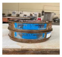
Fig 5. Sieves 1.18mm and 0.6mm
