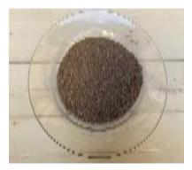
Fig 6. Prepared Sewage sludge (adsorbent).
