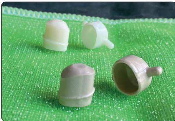
Fig. (2): Samples milled in the CAD-CAM machine from two disc materials (PEEK and GN CAD-CAM discs).
