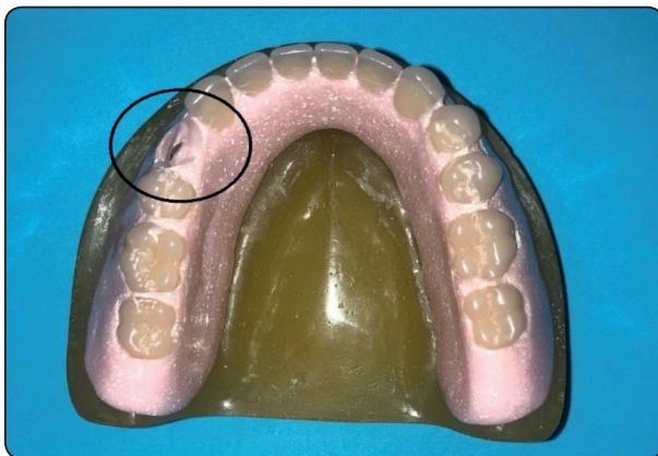
Fig. (4): Conventional acrylic resin Acrostone heat cured PMMA + 5% zirconium powder
