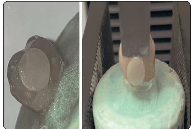
Fig. (1) Cemented ceramic disc on tooth surface before and during measurement.
