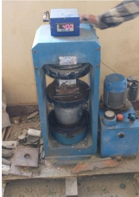
Fig.3: Compressive strength test procedure.
