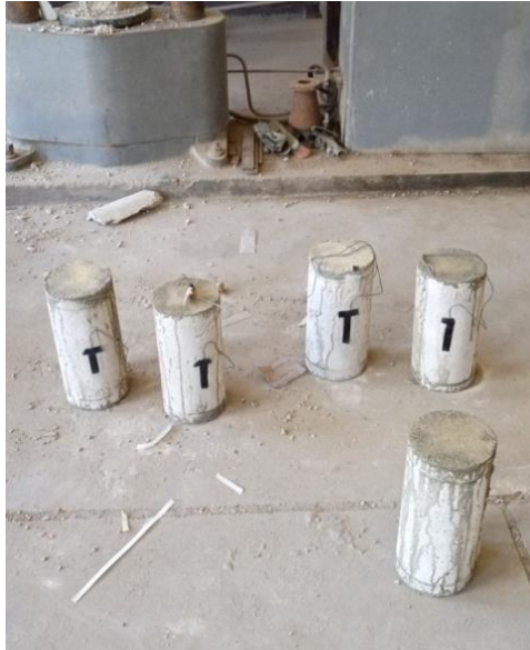
Fig.6: Showing the strain gauge used on the samples.
