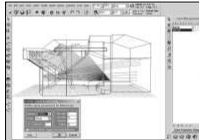
Fig. (5) An output of the Linked Acoustic Rays analysis from the Ecotect program
