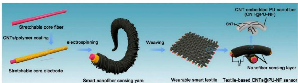
Fig. 4: Processes for fabricating carbon nanotube-encased nanofiber sensing yarn[29]
