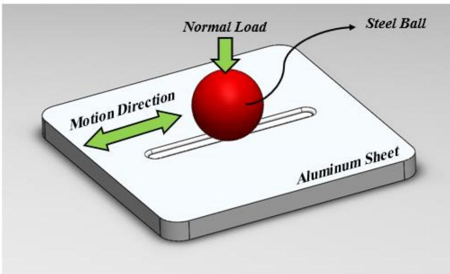
**Fig. 2** Details of the test process.
