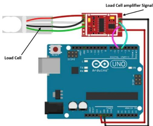
**Fig. 3** Wiring diagram for load cell Signal.
