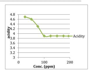
Figure(4): Relation between the concentration of polymer and acidity.
