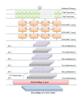
Fig. 2. CNN-LSTM/CNN-GRU NETWORK ARCHITECTURE
