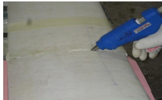
Fig. 3 Bonding two parts of wing
