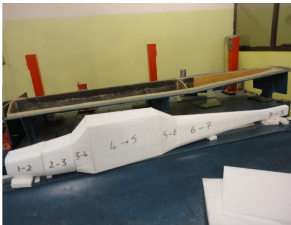
Fig. 4 Fuselage made of foam
