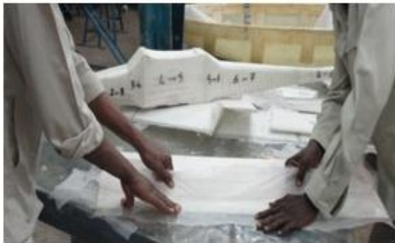
Fig. 2 Wing covering with fiber glass
