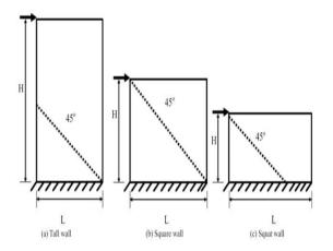
Fig.6. Direction of diagonal cracks in masonry shears walls [38].
