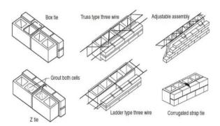
Fig.3. Joint Reinforcement Applications in Masonry
