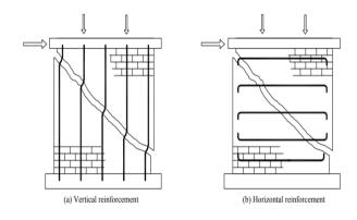
Fig.2. Role of reinforcement in resisting masonry shears Failure.
