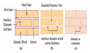
Fig.8. Modeling strategies of masonry structures: a) detailed micro-modeling; b) simplified micro-modeling; and c) macro-modeling [51].
