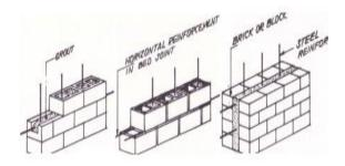
Fig.4. Placing of reinforcement in masonry
