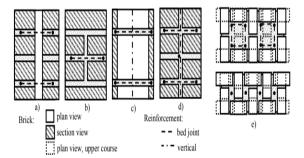
Fig.5. a) Reinforced cavity wall, b) Reinforced solid masonry, c) Reinforced hollow unit masonry, d) Reinforced grouted masonry, e) Reinforced pocket type wall.
