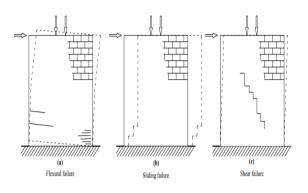
Fig.1.The failure modes of masonry wall [23].
