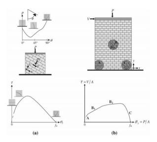
Fig.7. Failure modes and limit domains for masonry: a) Scale of the material; b) Scale of the pier from [41].
