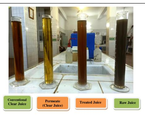
Figure (10): Clarified juice quality obtained by treatment of raw cane juice with organo- bentonite/ultrafiltration (organo-bentonite dose 0.5g/L) compared to conventional limed–sulfated clear juice.
