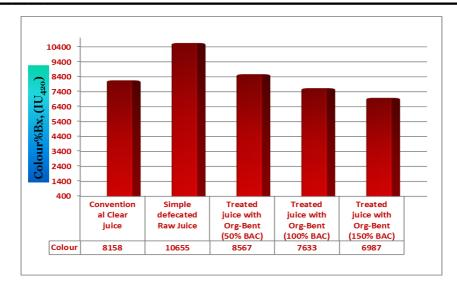
Figure (5): Effect of BAC concentration on colour adsorption of raw cane juice at constant temperature and pH.
