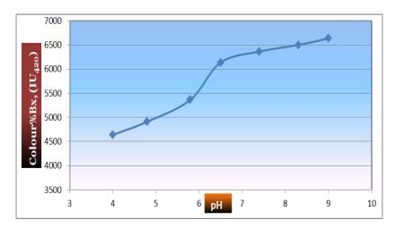
Figure (7): Effect of pH on colour removal from raw cane juice by modifiedbentonite at constant temperature.
