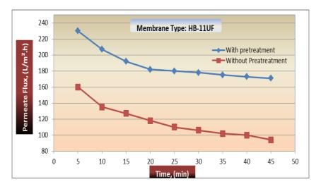
Figure (2): Effect of pretreatment of raw cane juice on flux during filtration of raw cane juice through HB-11UF membrane at pH 7.5, TMP 4 bar and temperature 45-50 °C.
