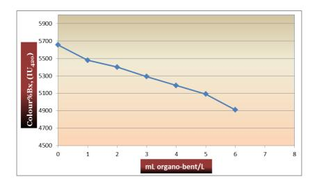
Figure (6): Effect of organo-bentonite dose on colour removal from raw cane juice by modified bentonite at constant temperature and pH.
