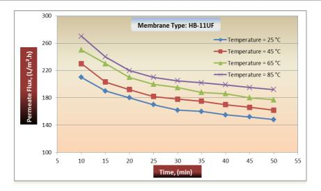
Figure (4): Effect of temperature on flux during filtration of raw cane juice through HB-11UF membrane at pH 7.5 and TMP 4 bar.
