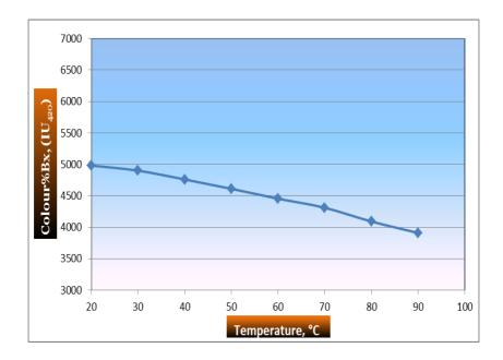
Figure (9): Effect of temperature on colour removal from raw cane juice by modified bentonite at constant pH and organo-bentonite dose 0.5 g/L.
