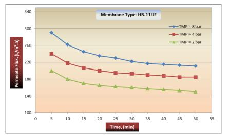
Figure (3): Effect of transmembrane pressure on flux during filtration of raw cane juice through HB-11UF membrane at pH 7.5 and temperature 45-50 °C.
