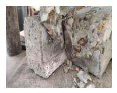
Fig. 12. Failure in case of nails
