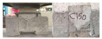
Fig. 10. Failure at the interface
