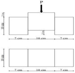
Fig. 4. Test sample dimensions
