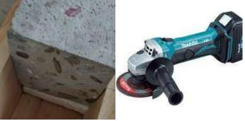
Fig. 1. Surface preparation by grinding
