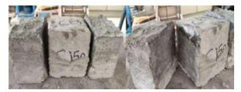
Fig. 11. De-bonding in case of epoxy resin
