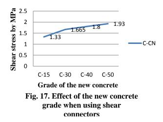
The test specimens were cast with shear connectors (one for each side) and without any adhesive agent. Using nails shows more bond strength at the interface when using a higher new concrete strength.
