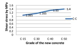
Fig. 15. Effect of the new concrete grade
