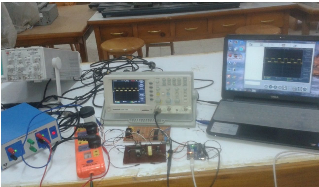
Fig. 10. Test setup of IH power supply system.
