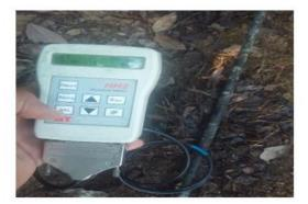
Figure 3. Moisture meter instrument type (HH2)
