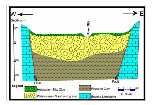
**Fig. 5:** Hydrogeological cross section for the area south of Assuit city (after Farrag, 1982).
