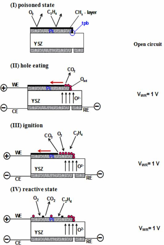
**Fig. 9:** Schematic drawing of the ignition mechanism as proposed by Toghan et al. for the electrochemical activation of catalytic ethylene oxidation on Pt/YSZ under UHV conditions. YSZ = yttria-stabilized zirconia, tpb = three-phase-boundary (solid electrolyte/metal/gas), WE = working electrode, CE = counter electrode and RE = reference electrode, from [92].
