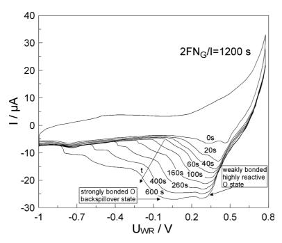
**Fig. 7:** Cyclic voltammograms (CV) of the Pt/YSZ catalyst electrode for various holing time at 673 K under UHV conditions, from ref. [84]. The Pt film was deposited on the surface of YSZ specimen using a thin coating of Pt paste followed by drying and calcination in air.
