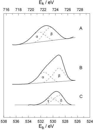
**Fig. 4:** Photoelectron spectra of the O 1s region of a porous Pt/YSZ catalyst demonstrating the effect of electrochemical pumping at 673 K. (A) Open-Circuit conditions, (B)  $V_{WR}$ = +1.2 V and (C) Difference spectrum of A and B, From ref. [79].
