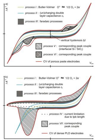
**Fig. 8:** Interpretation of CV peaks using different Pt/YSZ electrodes: (a) porous Pt film, and (b) dense Pt(111) film produced by pulsed laser deposition (PLD), according to ref. [85].
