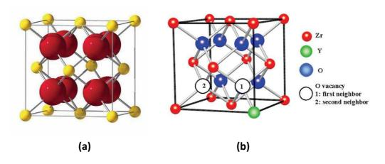
**Fig. 1:** (a) Cubic fluorite type structures of: (a) Zirconia (ZrO<sub>2</sub>) with the O ions shown in red circles and the smaller Zr ions shown in yellow, and (b) Yttrium stabilized zirconia (YSZ), adopted from references [33, 34].
