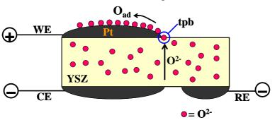
**Fig. 6:** Scheme showing the electrochemically induced spillover of oxygen ions onto the surface of the metal electrode. Oxygen ions are transported through the YSZ solid electrolyte during the anodic (positive) polarization of the metal catalyst (working electrode) and are discharged at the tpb and the discharged oxygen species then migrate onto the surface of the Pt electrode.
