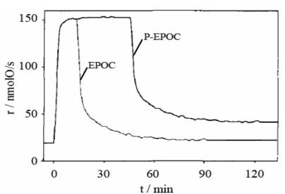
**Fig. 10:** A typical galvanostatic NEMCA experiment of ethylene oxidation at IrO<sub>2</sub>/YSZ catalyst due to current application (300  $\mu$ A) for two different polarization times: (a) short polarization to give reversible EPOC and (b) long polarization to give P-EPOC [93]. Experimental conditions: T= 380 °C, p(O<sub>2</sub>)= 17 kPa, p(C<sub>2</sub>H<sub>4</sub>)= 140 Pa, reproduced with permission from Springer.
