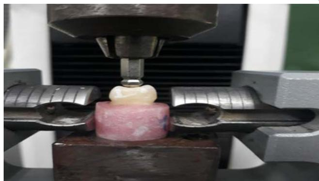
**Figure 3:** Inlay restorations under load in the Universal Testing Machine
