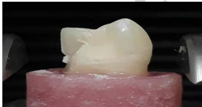
**Figure 4:** Fractured inlay restoration from group A showing catastrophic failure
