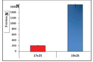
Fig. (6) Effect of coating on friction of coated 0.017 x 0.025" wire in 0.018" bracket slot size and coated 0.019 x 0.025" wire in 0.022" bracket slot size.
