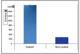
Fig. (5) Bar chart showing the effect of coating on friction of 0.019 x 0.025" stainless-steel wire in 0.022" bracket slot size.
