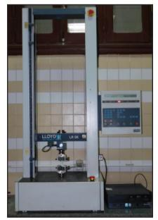
Fig. (2) The LR5K Lloyd universal testing machine.
