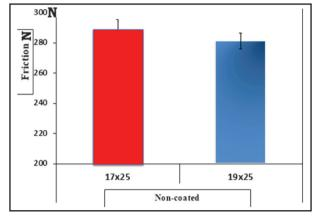
Fig. (7) Effect of friction of 0.017 x 0.025" wire in 0.018" bracket slot size and 0.019 x 0.025" wire in 0.022" bracket slot size.
