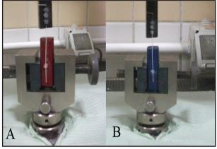
Fig. (3) A: Testing the friction of 0.017 x 0.025" arch-wires in 0.018" bracket slot size. B: Testing the friction of 0.019 x 0.025" arch-wires in 0.022" bracket slot size.
