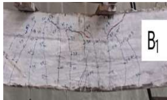
(b) Experimental crack pattern.
