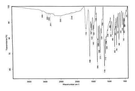
Figure (14): FT-IR spectrum of methyl red.
