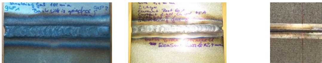
Fig. 1. Welding regions produced by TIG welding (left), Plasma welding (middle) and Laser welding (right).
