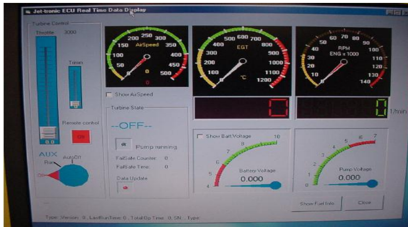
Fig. 8. Engine control panel screen
