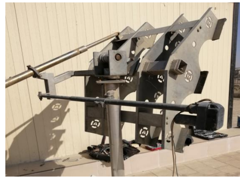
Fig.4 Linear actuator driven small sized heliostat 1m 2
