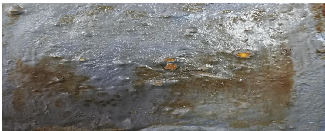
Fig. 20. Corrosion inhibitor A sample with two shells after scratching – after immersing in 10% sulfuric acid after one year
