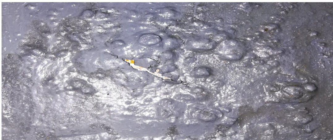
Fig. 22. Corrosion inhibitor B sample with one shell after scratching – after immersing in 10% sulfuric acid.
