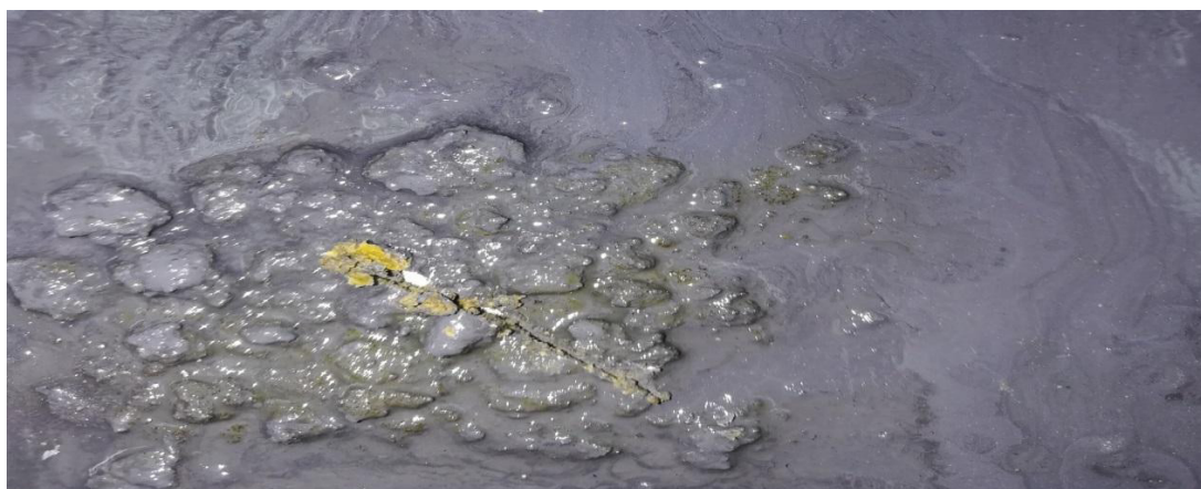
Fig. 15. Corrosion inhibitor A sample with one shell after scratching – before immersing in 10% sulfuric acid.
