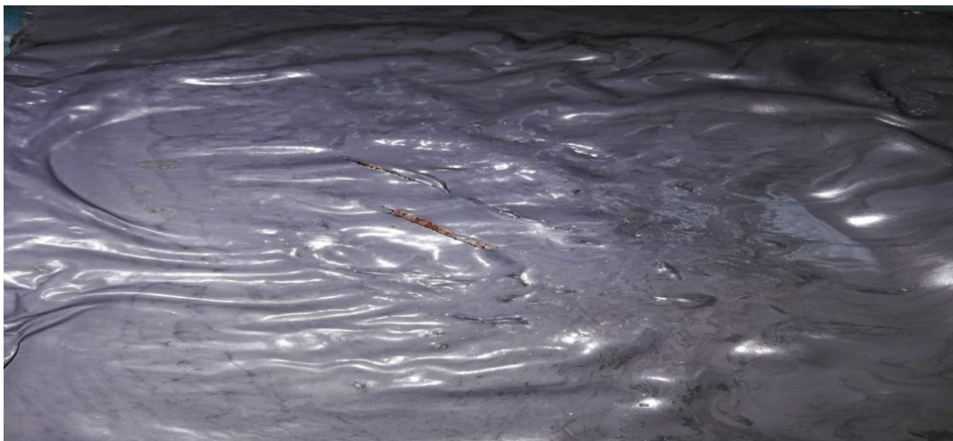
Fig. 7. Chema-poxy sample after scratching and immersing in 10% sulfuric acid for 48 hours.
