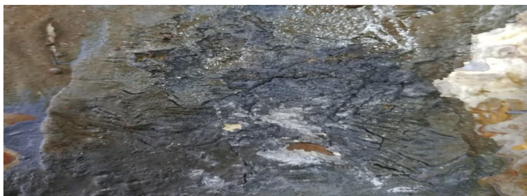
Fig. 26. Corrosion inhibitor B sample with two shells after scratching – after immersing in 10% sulfuric acid after one year.
