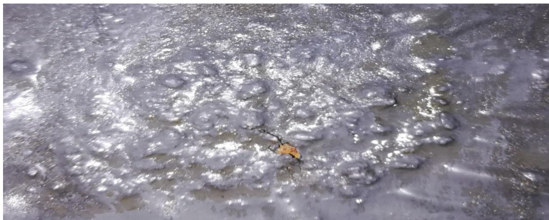
Fig. 10. linseed sample with one shell after scratching – after immersing in 10% sulfuric acid for 48 hours.
