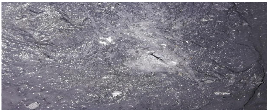
Fig. 24. Corrosion inhibitor B sample with two shells after scratching – before immersing in 10% sulfuric acid.
