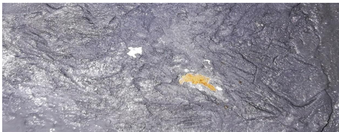
Fig. 25. Corrosion inhibitor B sample with two shells after scratching – after immersing in 10% sulfuric acid.
