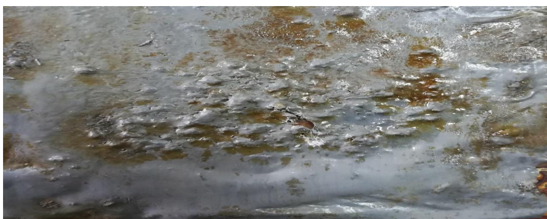
Fig. 11. linseed sample with one shell after scratching – after immersing in 10% sulfuric acid after one year.
