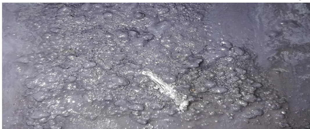
Fig. 12. linseed sample with two shells after scratching – before immersing in 10% sulfuric acid.
