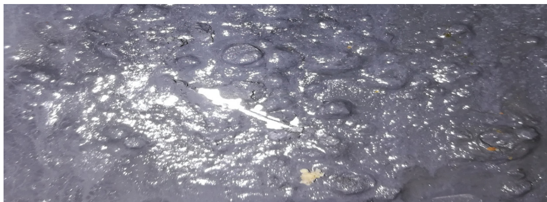
Fig. 21. Corrosion inhibitor B sample with one shell after scratching – before immersing in 10% sulfuric acid.
