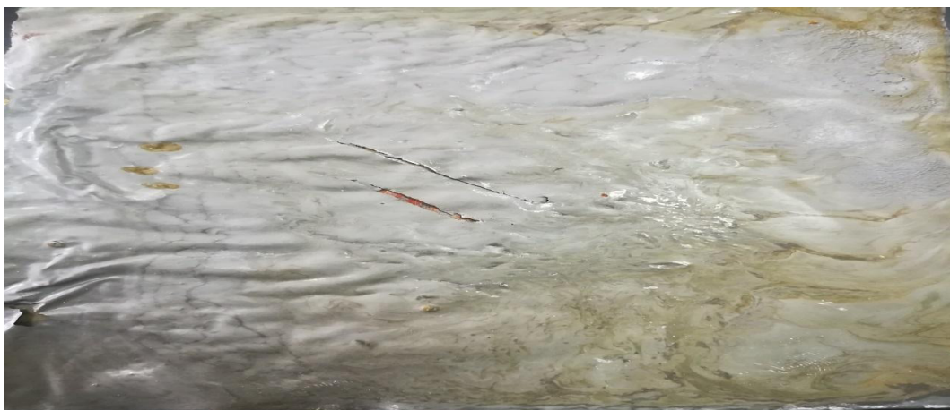
Fig. 8. Chema-poxy sample after scratching and immersing in 10% sulfuric acid after one year.
