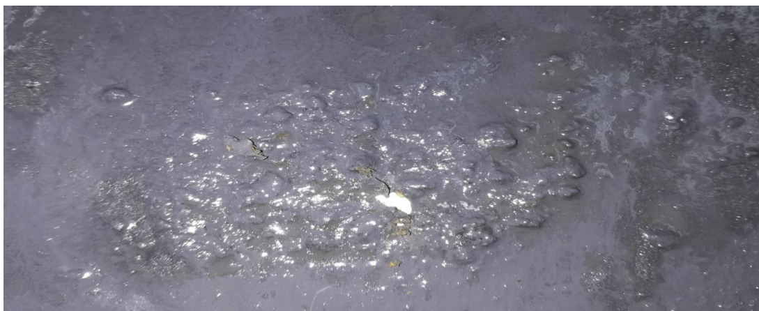
Fig. 9. Linseed sample with one shell after scratching – before immersing in 10% sulfuric acid.
