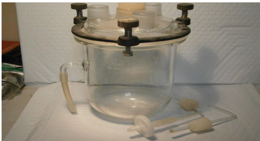
Fig. 1. Four necked glass kettle for preparation.
