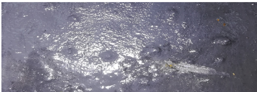
Fig. 18. Corrosion inhibitor A sample with two shells after scratching –before immersing in 10% sulfuric acid.
