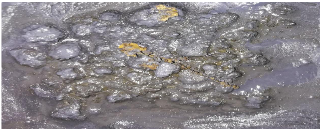
Fig. 16. Corrosion inhibitor A sample with one shell after scratching – after immersing in 10% sulfuric acid.
