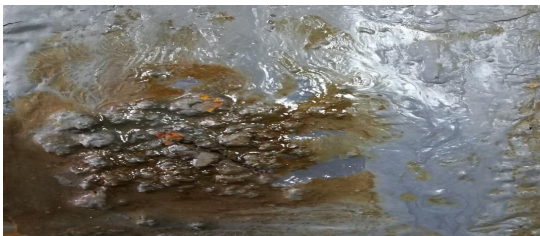
Fig. 17. Corrosion inhibitor A sample with one shell after scratching – after immersing in 10% sulfuric acid after one year.
