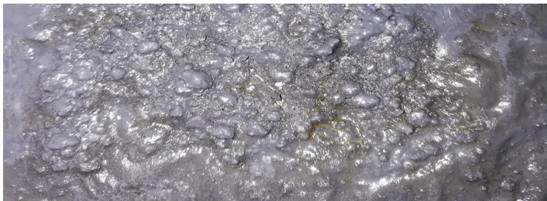
Fig. 13. linseed sample with two shells after scratching – after immersing in 10% sulfuric acid for 48 hours.
