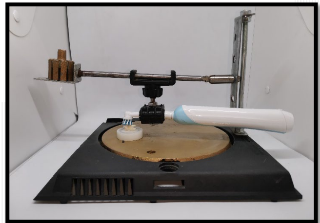
Figure 2: photograph showing the load fixation device with the electric toothbrush fixed to it.
