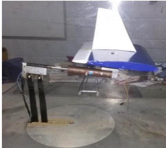
Fig. 3. BlueBird MAV during aerodynamics measurements
