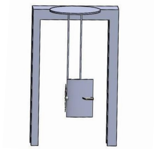
Fig. 7. Bluebird on mass moment of inertia test rig
