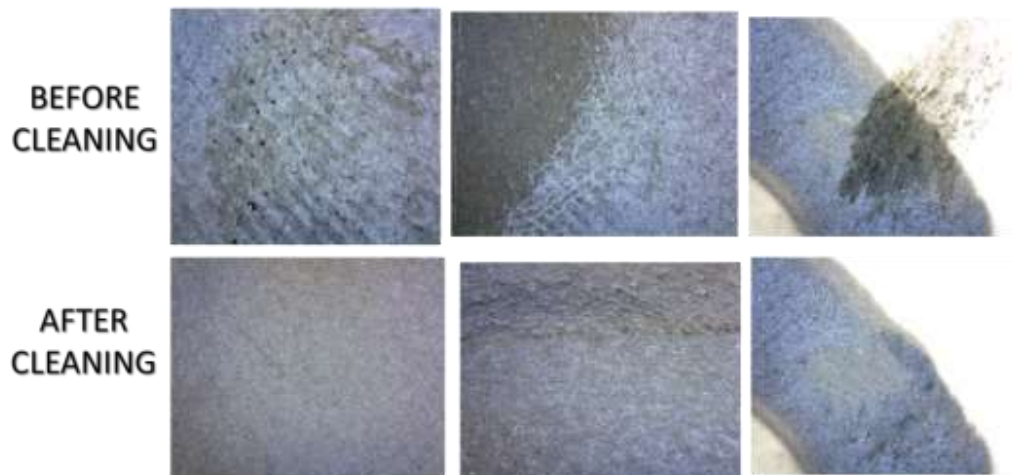
Fig. 19. Microscopic inspection of silver mirroring removal using vinyl eraser.
