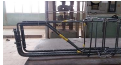
Fig.1 .e: spliced tying type-2 rows
