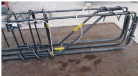
Fig.1. d.: spiral spliced type of tying- 2 rows
