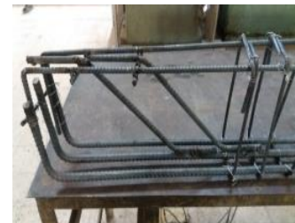
Fig. 1. c.: Welded tying type.
