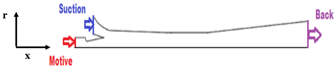
Fig. (1) Diagram of computational domain of ejector steam flow [4,10]
