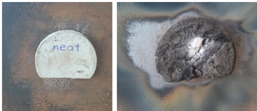
Figure 8 Neat sample before and after Oxy-acetylene torch test
