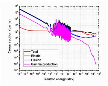
Fig. (1): U-235 cross-section [21].
