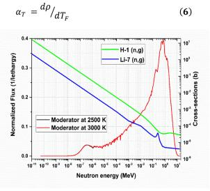
Fig. (10) Flux behavior with moderator crosssection
