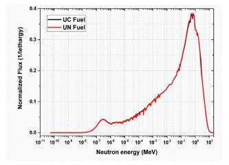
Fig. (6): Flux distribution for ZrH<sub>1.8</sub> moderator with UC and UN fuel
