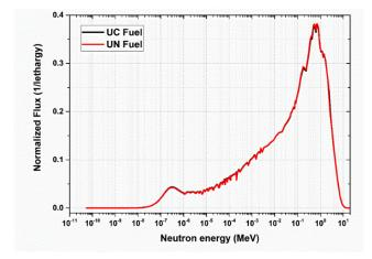
Fig. (5): Flux distribution for LiH moderator with UC and UN fuel
