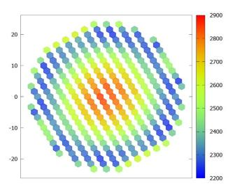
Fig. (11): Outlet temperature distribution for the propellent at each fuel element
