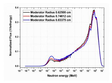
Fig. (7): Flux distribution for various moderator radius
