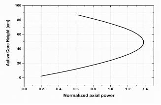
Fig. (9): Axial power distribution
