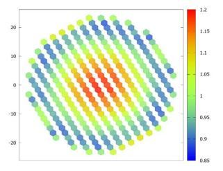
Fig. (8): Radial power distribution
