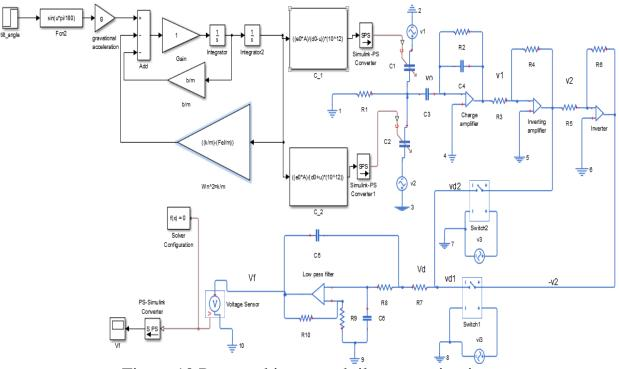
Figure 10 Proposed integrated tilt sensor circuit
