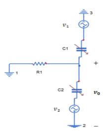
Figure 5 Variable capacitors for tilt sensor
