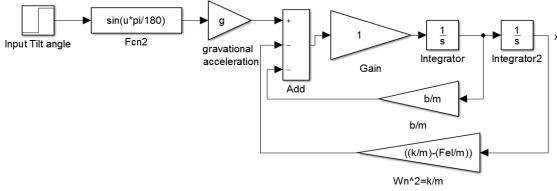
Figure 4 Tilt sensor mechanical part model
