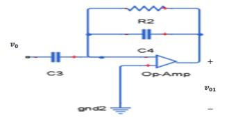
Figure 6 Charge amplifier  $v_{01}(s) = -v_0(s) \frac{sC_3R_2}{1 + SC_4R_2}$  (4) The inverting amplifier is used to amplify and invert the applied input signal to it as
